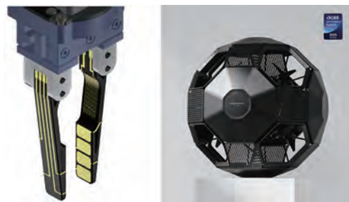
The MoR ™ multifunctional robotic finger (left) and the HAGAMOSphere ® omnidirectional multicopter
