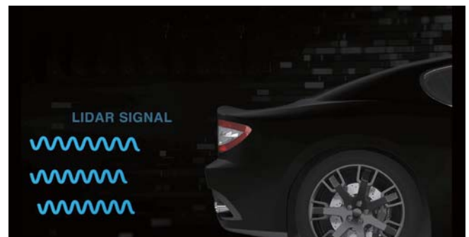
The NIR wavelengths of LiDAR signals are absorbed by the carbon black pigment of automotive coatings, significantly hindering signal response.
