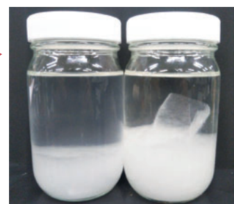
Paper coated with HYDRECT dissolves completely in chemicals (left), while that laminated with polyethylene does not (right)
