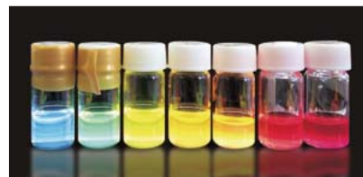
Colloidal QD dispersions irradiated with a UV light
