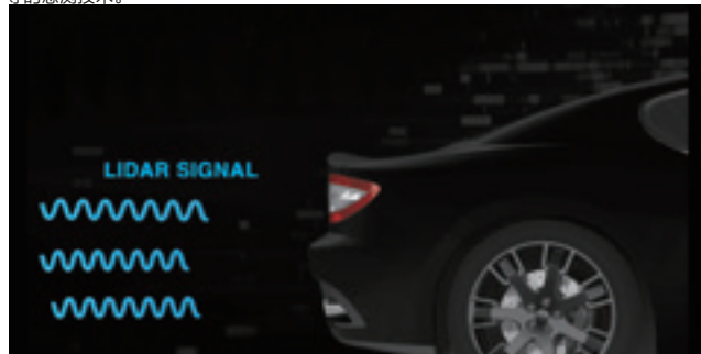
LiDAR信号的近红外光被外漆的碳黑颜料吸收，信号响应性显著降低
